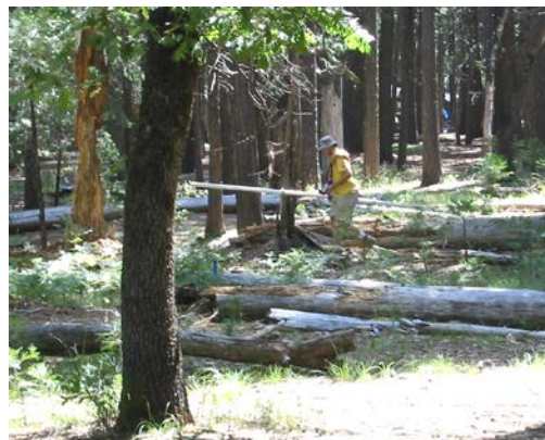
Technician acquiring ground conductivity data using a Geonics EM-31 terrain conductivity meter
